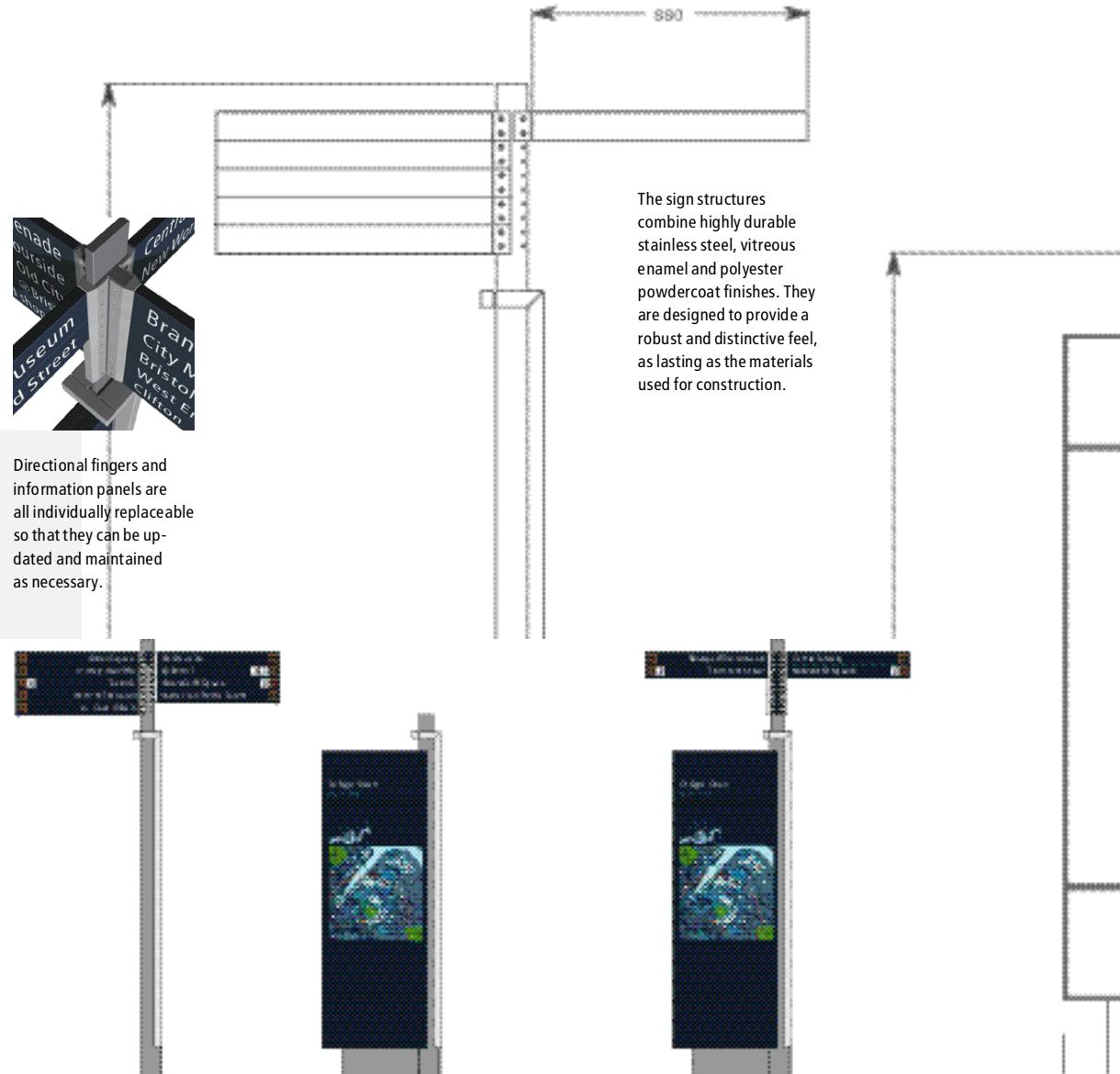
The sign structures combine highly durable stainless steel, vitreous enamel and polyester powdercoat finishes. They are designed to provide a robust and distinctive feel, as lasting as the materials used for construction.
